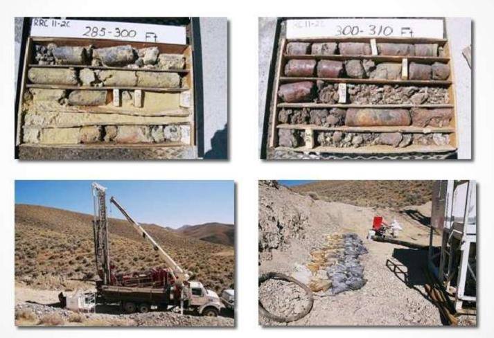
Reverse circulation drill Rig which produces bags of sample chips
